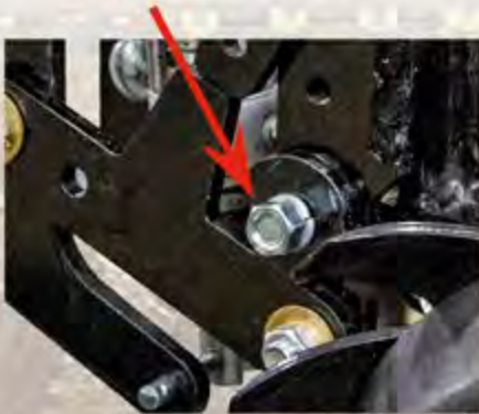
5 Sided Cam is easily adjustable with a 3/4" Wrench
